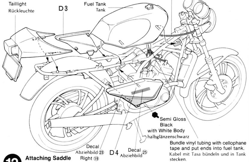
Put the end of the tubing into fuel tank.
