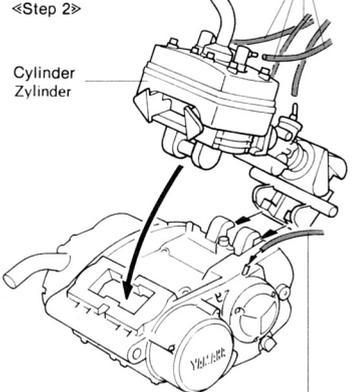
**3** Placing Engine into Frame
