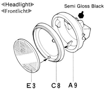
Before cementing plated parts, remove plating with a knife etc. from the surface to which cement is applied.
